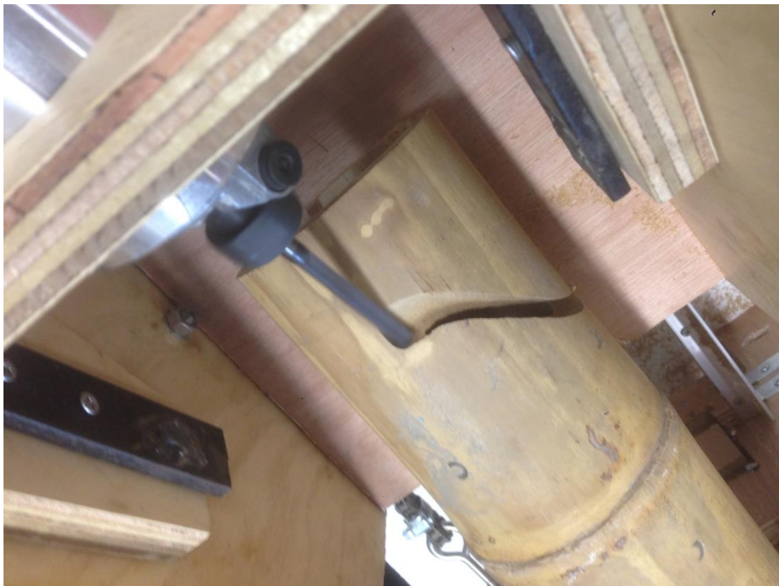
Figure 12 – Image of the digital fabrication too milling a ‘fish mouth’ joint
