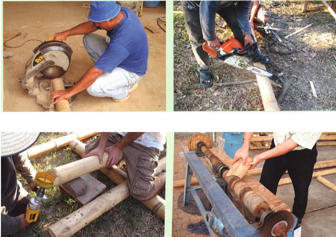
Figure 9 - Types of tooling used in the fabrication of joints. Note the lack of precision in the jigs and the reliance of the user to ‘eye’ out the accuracies. Image source Gernot Minke
