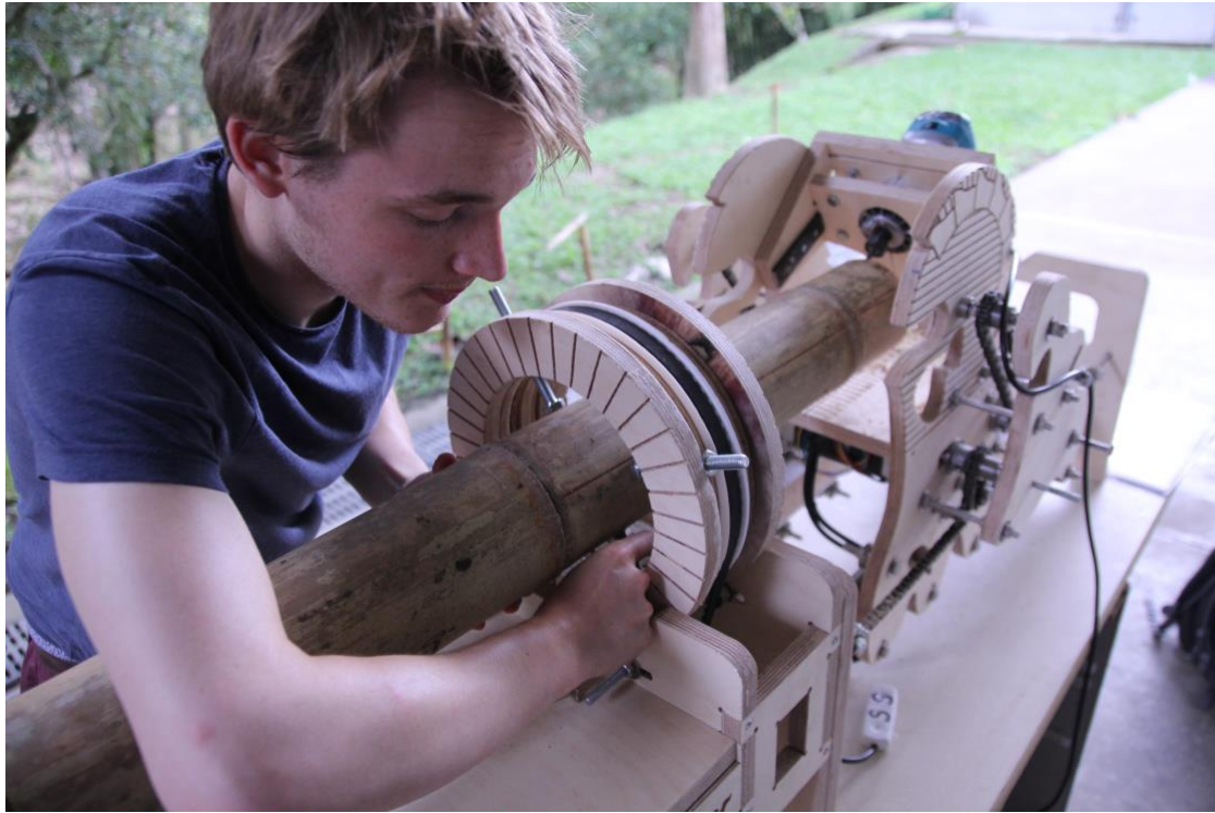
Figure 10 – Image of the 3 axis digital fabrication CNC tool with mounted bamboo.
