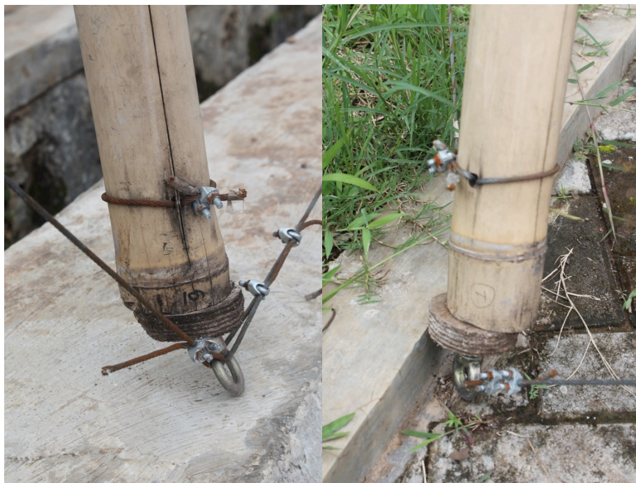
Fig. 11. Deformations at the bottom end of the legs.
