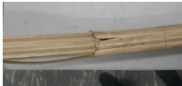
Figure 6 Bending test – bamboo laminate specimen.
