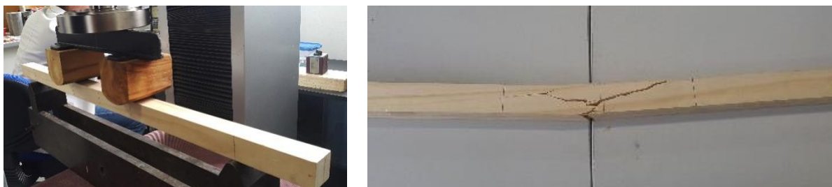
Figure 9 Bending test – radiate pine specimen.
