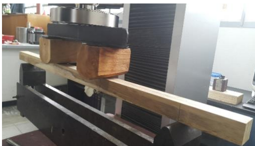
Figure 6 Bending test – bamboo laminate specimen.
