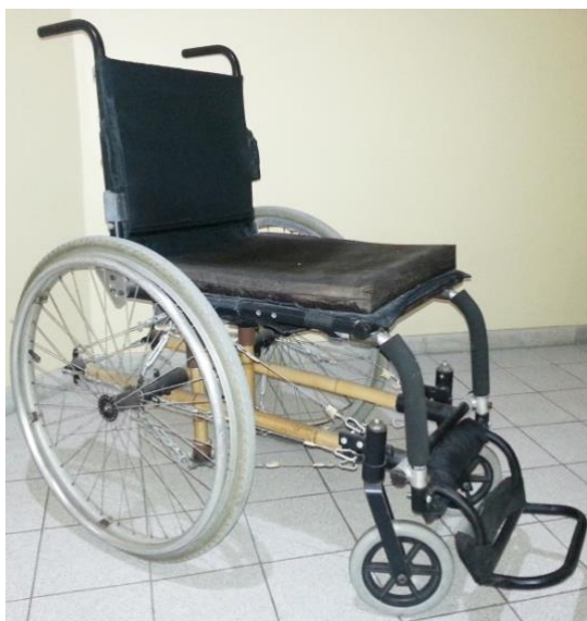
Figure 19. Test model of the wheelchair of tensegrity structure - prepared by author
