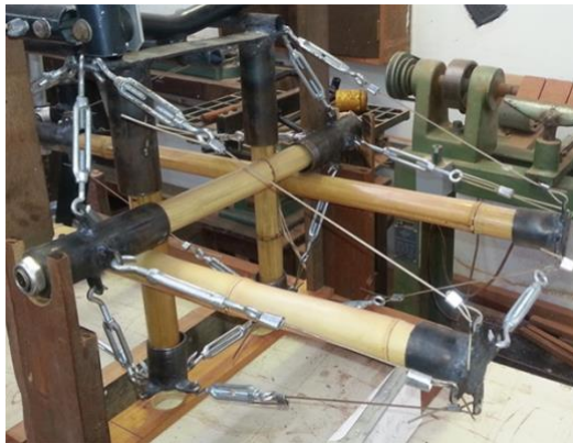
Figure 18. Gauge mounted with metal rods and connections and tensegrity structure wired (by author)
