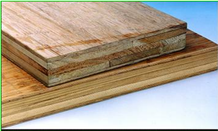
Wood-bamboo laminated veneer lumber
