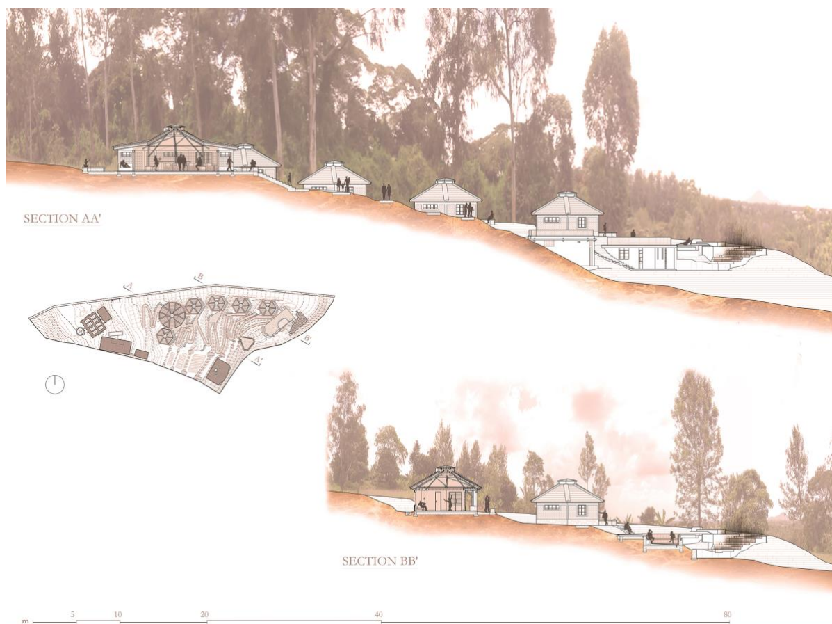
Figure 6: Sections of the proposal to note adaptation to the slope and intimate relation with the rainforest.
