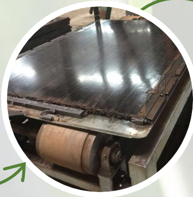
Fused with thermal-press into panels
