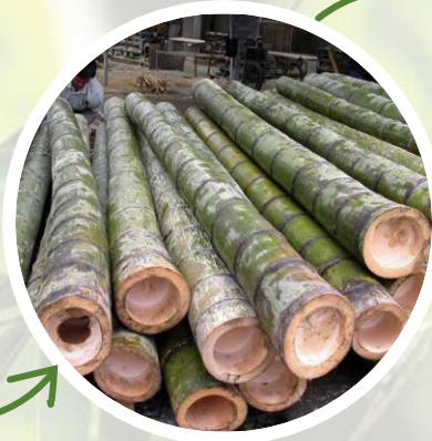
Culms cut to length of 6 1/2ft (2,000mm)
