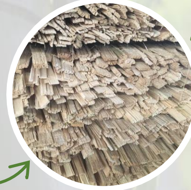
Stripes crush into strand of 1/64" (3mm) diameter
