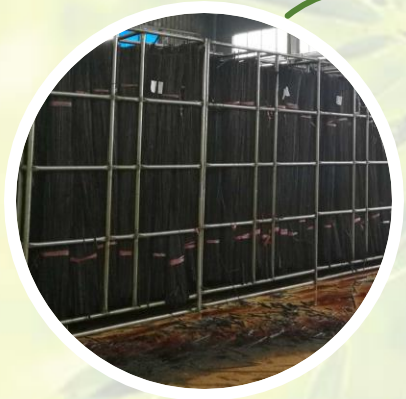
Binder Impregnation (meaning soak in binder thoroughly)
