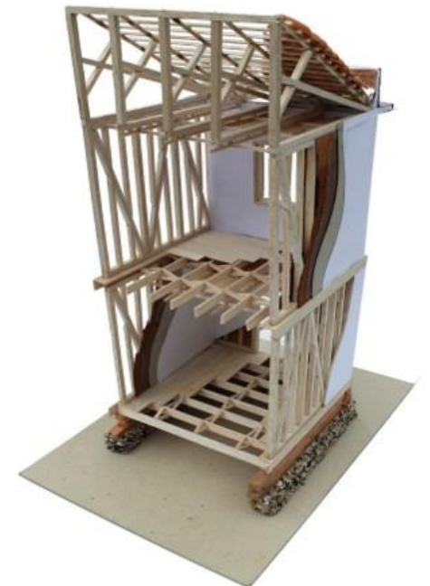
4- BAHAREQUE ENCEMENTADO CEMENTED BAHAREQUE
