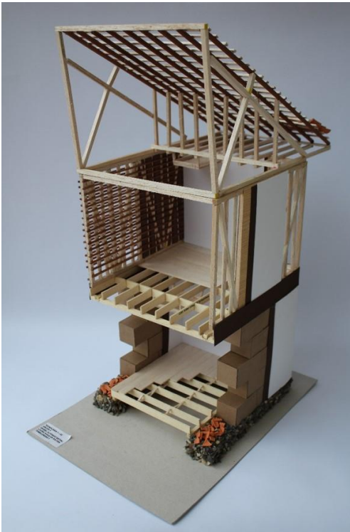
1- MAMPOSTERIA TAPIAS BAHAREQUE DE TIERRA RAMMED EARTH MASONRY CLAY BAHAREQUE
