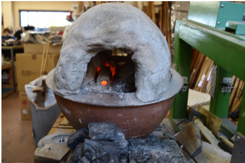
Figure 3. Oven to straighten Japanese arrow bamboo.
