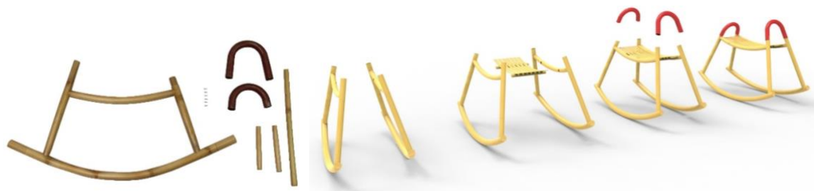
Figure – 08 – the components and the assembly of the rocker
