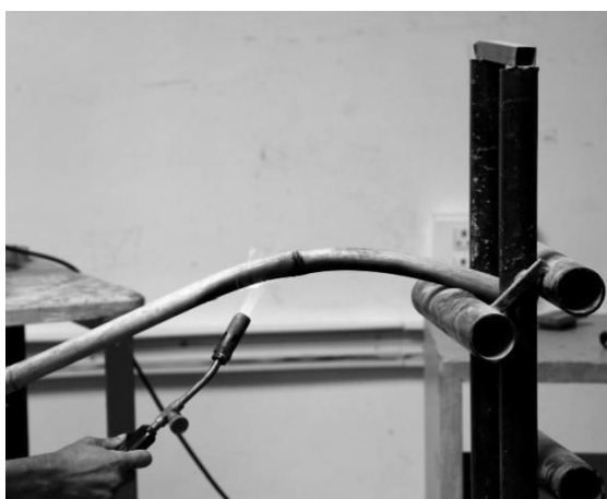
Figure – 03 – heat bending of solid bamboo
