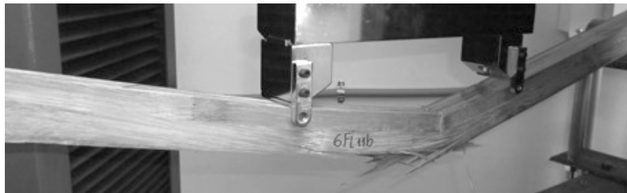
Figure 11. Sample 6FL11b at the end of the test
