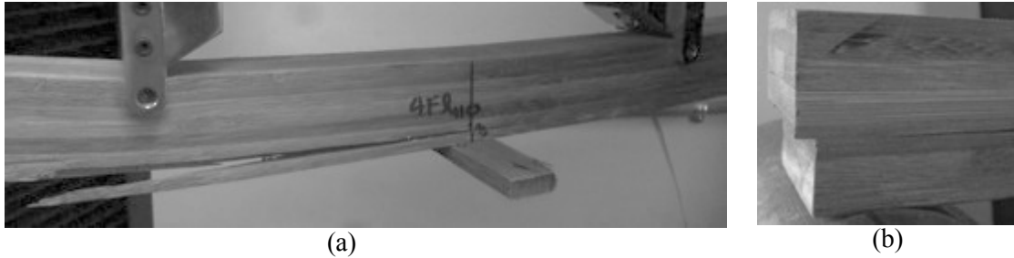
Figure 10. Sample 4FL11a: (a) tension crack and (b) shear failure near the support
