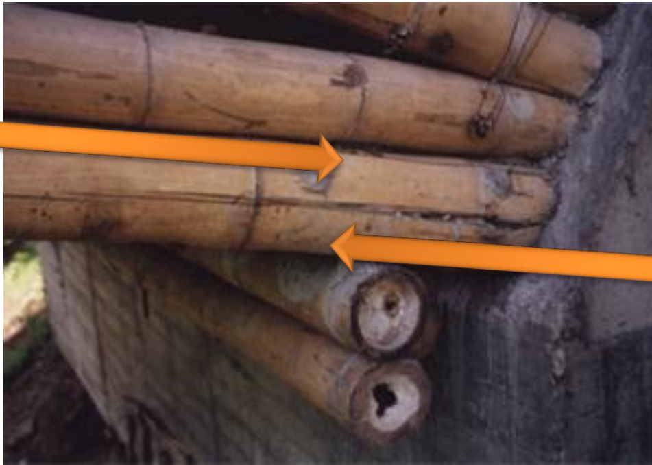
Shear failure of a bamboo culm along the direction of the fibres
